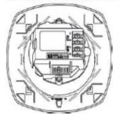
Adjust brightness by turning dial with screwdriver. Candela selection is displayed on front of unit.
