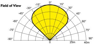
To meet the requirements of EN54:10 clause 5.4, where the ratio of the response points Dmax: Dmin should not exceed 1.41, the horizontal and vertical viewing angles max should not exceed
