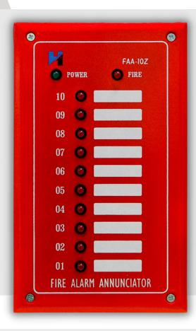
FAA-06/20Z is a conventional annunciator is designed to work with any Himmax Fire Alarm Control Panel. Auxilliary Panel Annunciator provides which zone should be given immediate attention. Annunciator operates when an alarm condition occurs, the zone indicator will flash and tone alert will continuously sound to alert everyone in the designated area. Annunciators should be located strategically so it can easily be heard and seen.
